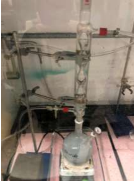
Figure 2. Stress corrosion cracking testing apparatus with hot-plate and condenser.
