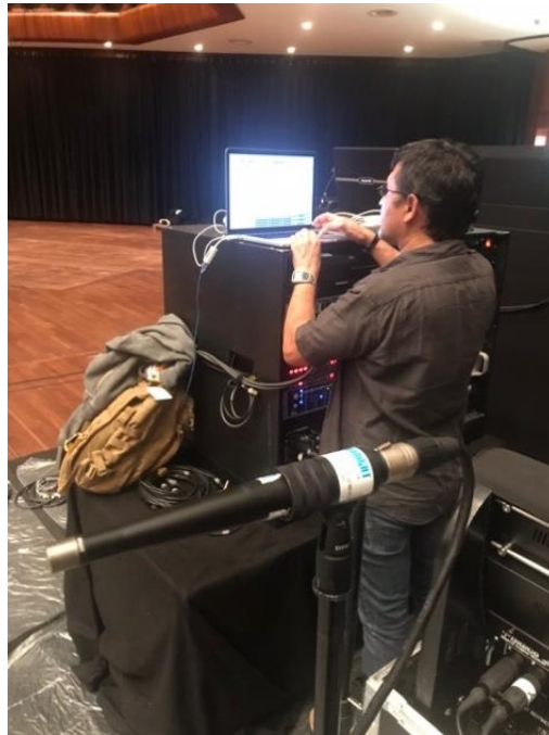
Figure 4.12: Mauricio Ramirez using SIM interface on Macbook Pro during tuning of Stravinski Auditorium, Montreux, Switzerland. He is positioned at the front-of-house mix position. Notice the SIM measurement microphone in the foreground. Photo by Tom Wetmore.
