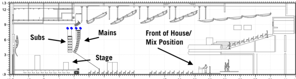
Figure 4.10: Plan view diagram of Stravinski Auditorium, showing some of the speakers and speaker groups (mains, flown subs), the stage, and the front of house (FOH) mixing position.
