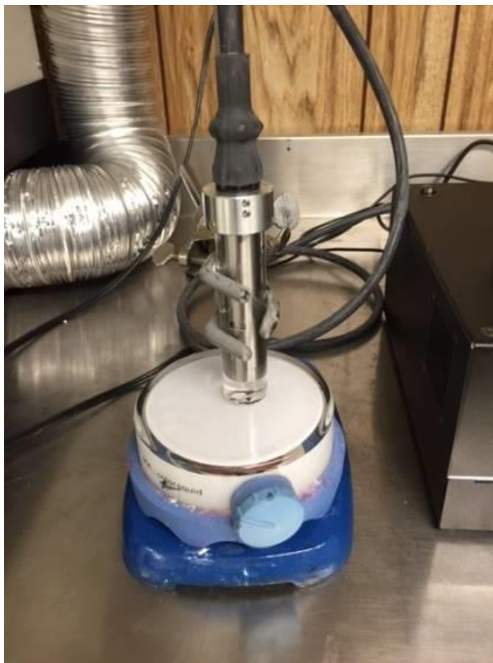
Figure 3 - Setup for Non-Aqueous Conductivity Measurements: Mixing was provided by a magnetic stir-bar to ensure homogeneity of the solution. A narrow vial was used to hold sample, allowing part of the Conductivity probe to serve as a cap to the sample chamber, preventing evaporation or effects caused by vapor pressure.
