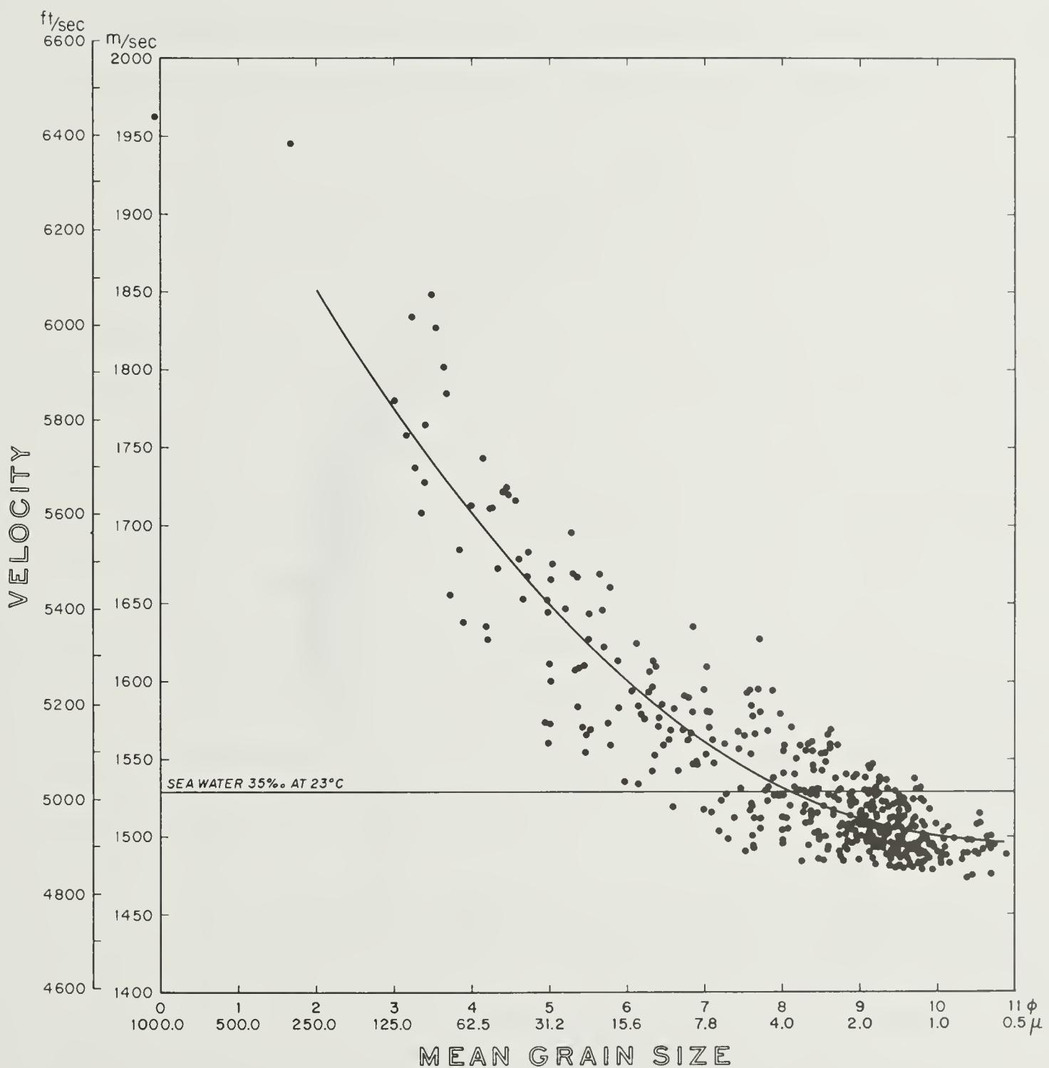
Figure 2. Mean grain size of unconsolidated deep-sea sediments plotted against sound velocity through sediment.
