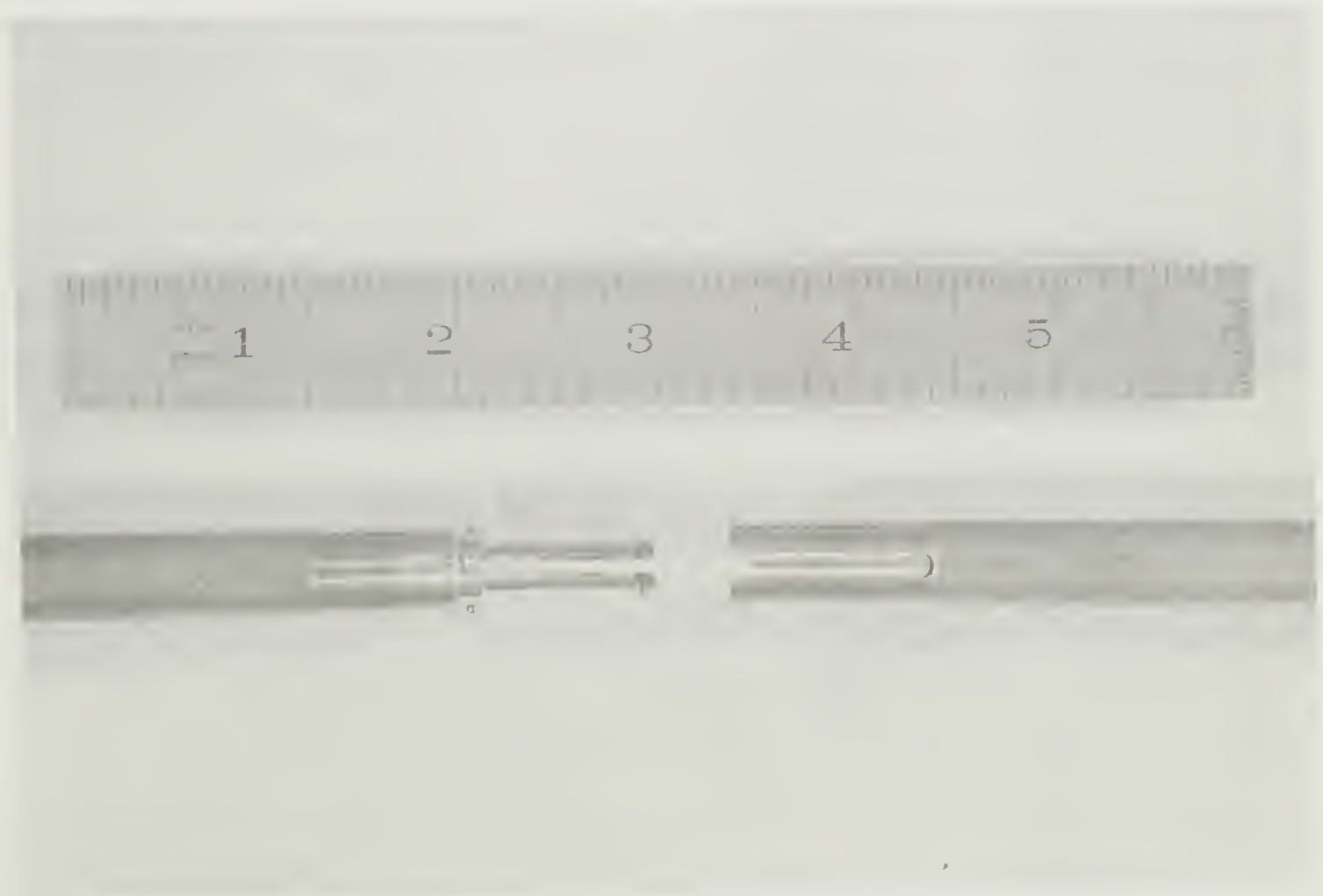
FIG. 14 - The knuckle joint, core liner tube on left and core lock on right. FIG. 15 - Locking joint of Emplacement Retrieval Tool. This joint transmits tension compression and torque.
