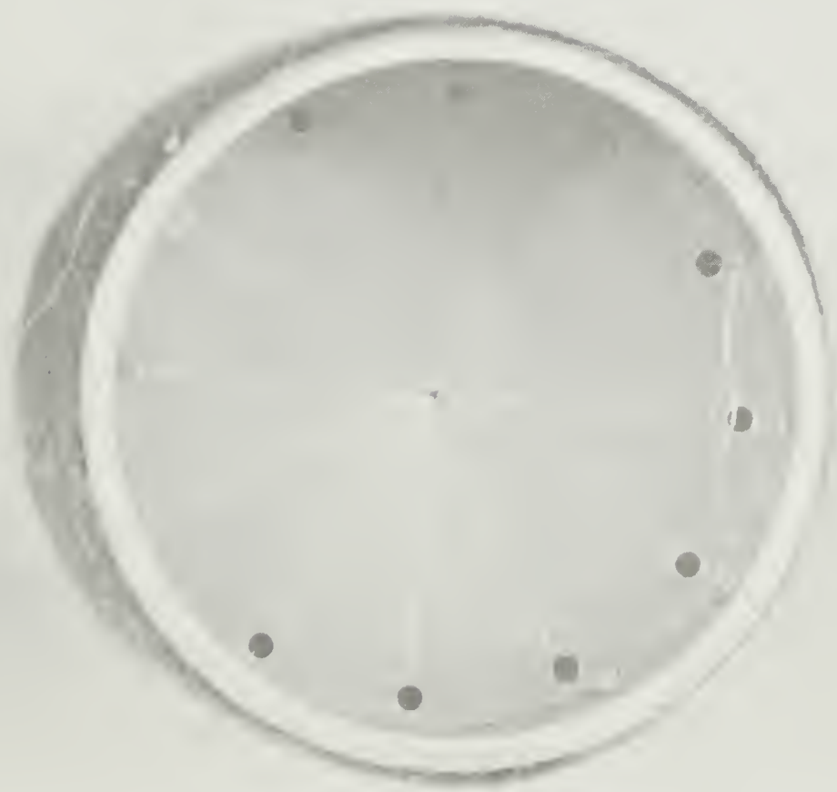
FIG. 9 - The felt flocked paper seal which prevents entry of rock particles into the core liner - drill stem interface.
