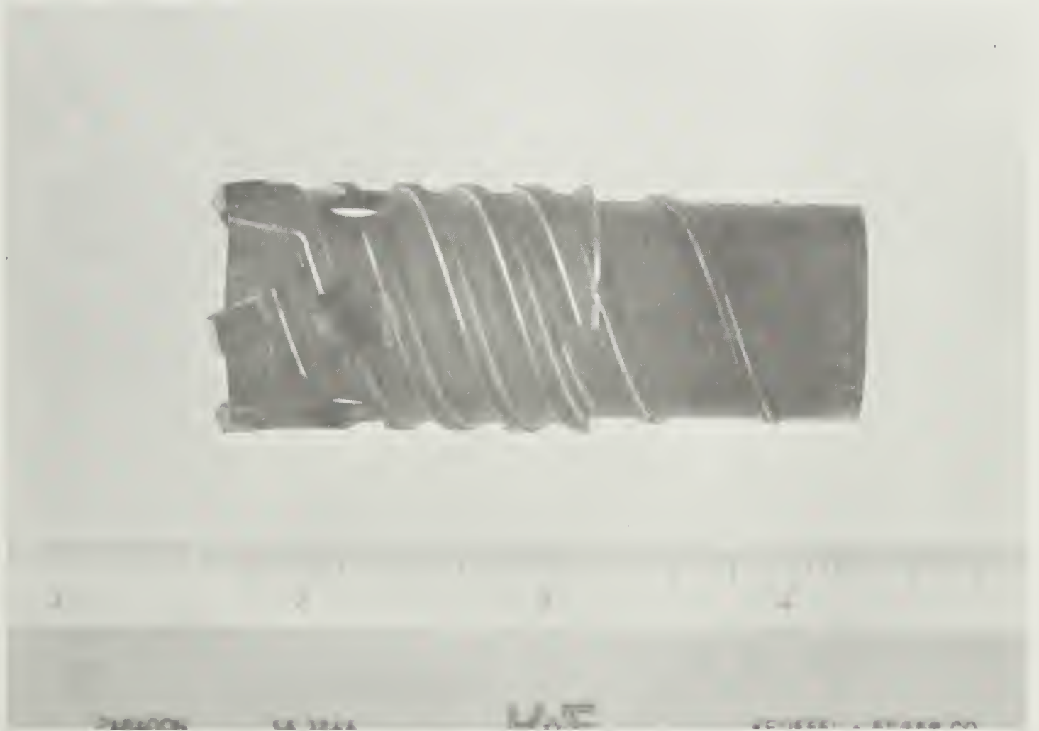
FIG. 6 - Prototype of solid faced drill bit. Note the core cutter protruding beyond the kerf cutter at left.
