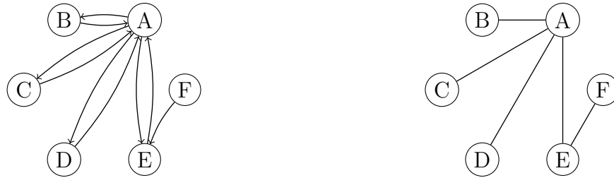
Figure 1.1: Example of a directed graph G (left) and the associated undirected graph H (right)
