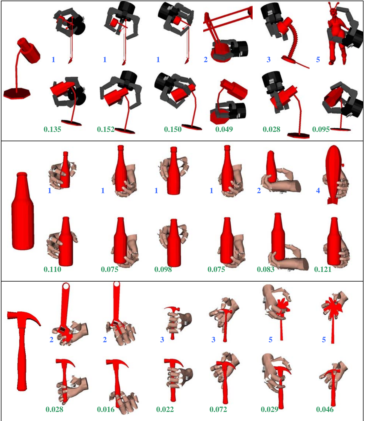
Fig. 2. Three example models and their grasps, using the database-backed planner with Zernike neighbors. For each model \alpha (left), the top row of images shows a neighbor n_k from the database, the value of k , and a pre-computed grasp on that neighbor. Directly below each neighbor is the same grasp executed on \alpha , along with its GWS epsilon quality measure.
