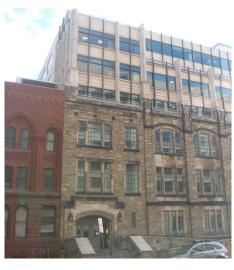
figure 29. Greene Building facadism (K.Wood)
