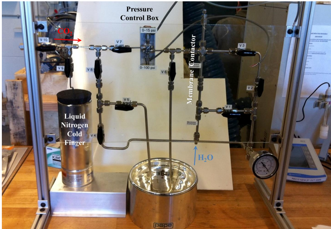
Figure 15: Initial construction of membrane system, showing the membrane contactor, pressure control box, liquid nitrogen cold finger, CO 2 and H 2 O flows.
