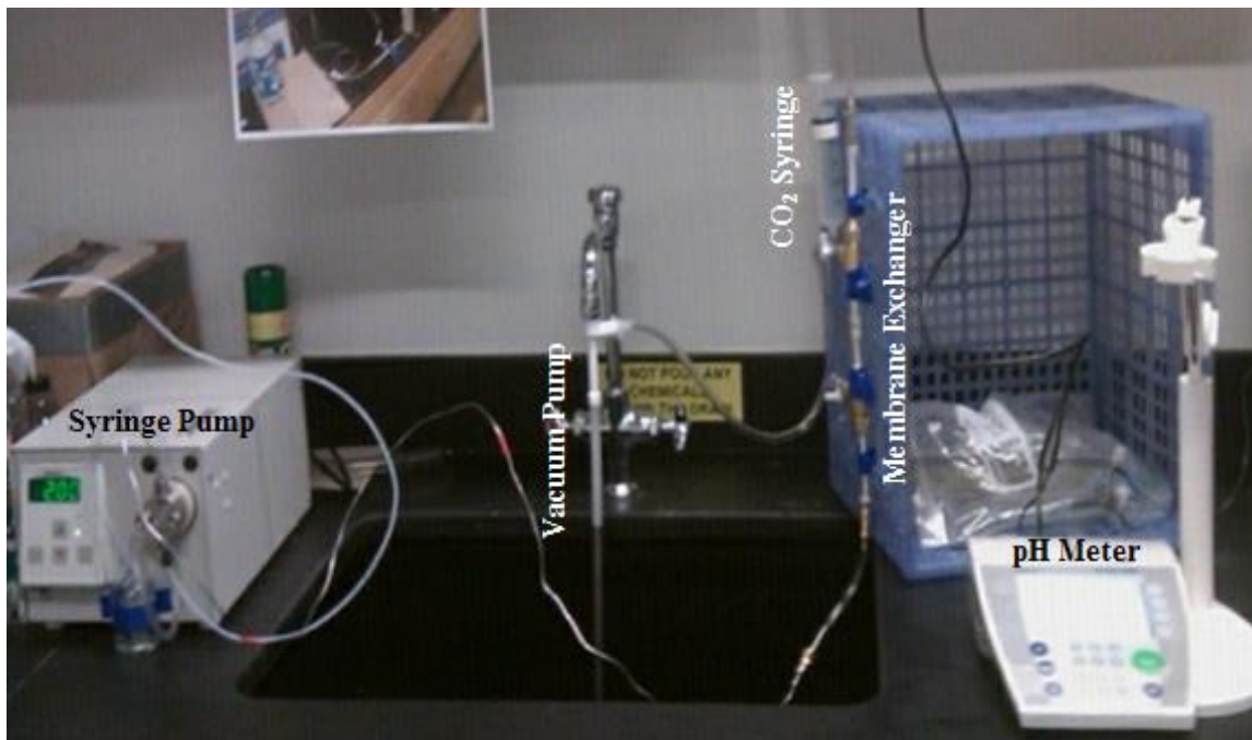
Figure 8: A picture of the initial testing setup with a vacuum pump and a CO 2 syringe connected to the membrane exchanger, a syringe pump for water inlet injection, and a pH Meter for outlet solution pH value measurement.
