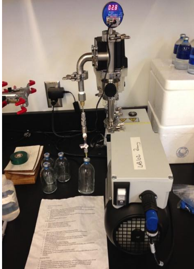
Figure 34: Setup of C14 sample bottle evacuation before CO 2 sampling.
