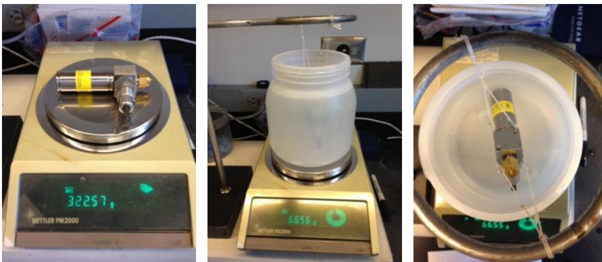
Figure 38: Archimedes' principle experiment to determine the internal volume of the cartridge.
