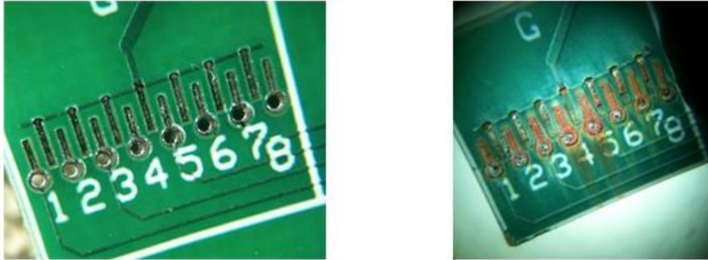
Figure 30: Comparison between new and corroded electrodes.
