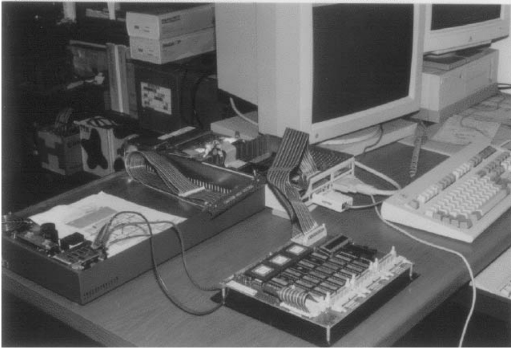
Figure 15: Interconnection between the Isoswitch and the host machine.
