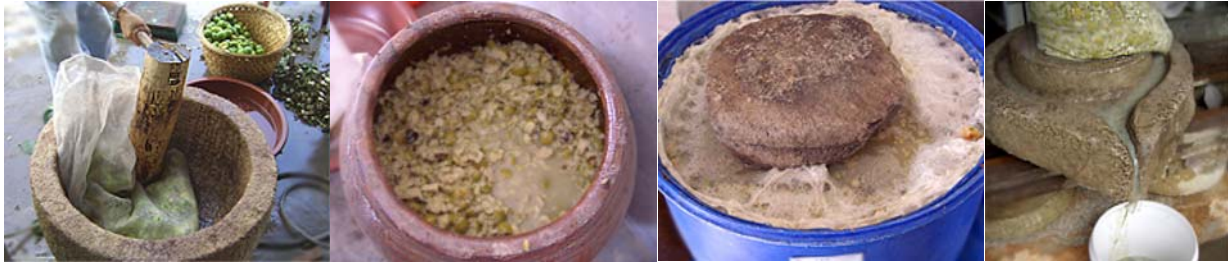
Figure 4. Kakishibu process, from crushing the immature persimmons (i) to its soak in water (ii) and week or more fermentation (iii) before being squeezed for the raw juice (iv) that will age to become Kakishibu
