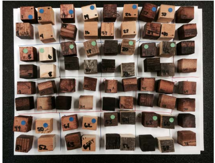
Figure 5. Treated 19mm cube samples arranged by jar number. Excluding the last row to the right, each set of four is (clockwise from upper left) kakishibu, raw juice, copper naphthenate, and untreated.
