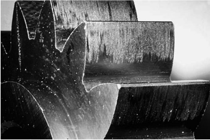
Fig. 18.22 Gear tooth surfaces with scuffing damage, from [67]
