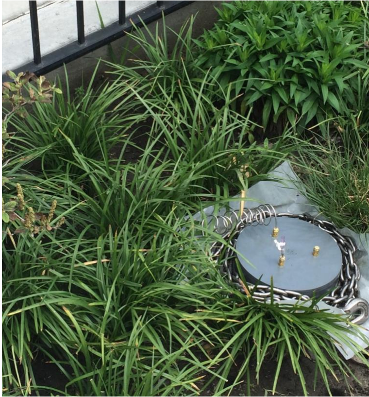
Figure 3.2 Static gas chamber for soil gas emissions sampling at two NYC rain gardens
