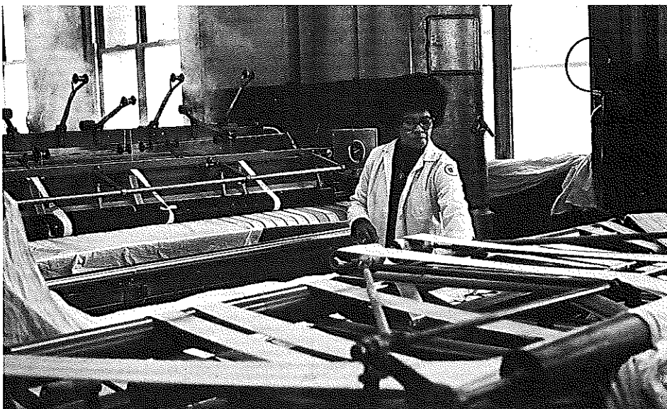
A hospital laundry worker operates a machine that folds and dries linen.
