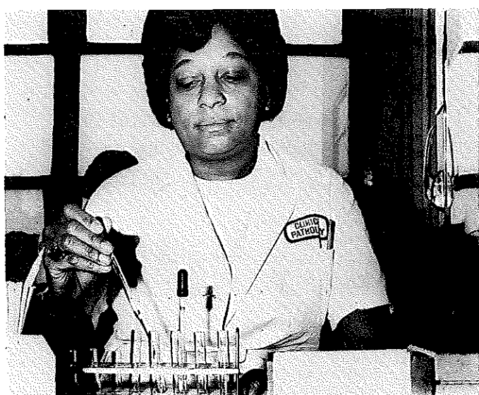
This lab worker is correctly pipetting by hand and is using a test tube rack. Use of the rack decreases the chance of spreading infection from lab spills.
