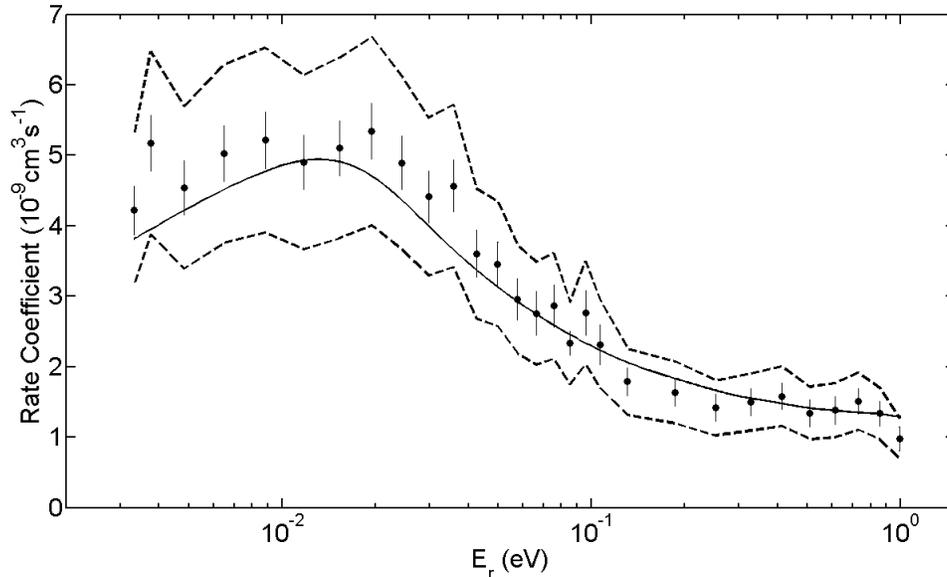
Fig. 1.— Our measured rate coefficient for reaction (1) from Kreckel et al. (2010). The circles show our measurements, the error bars are the  $1\sigma$  statistical uncertainty, and the dashed lines are the  $\pm 1\sigma$  total experimental uncertainty. The solid line is the theory of Čížek et al. (1998).
