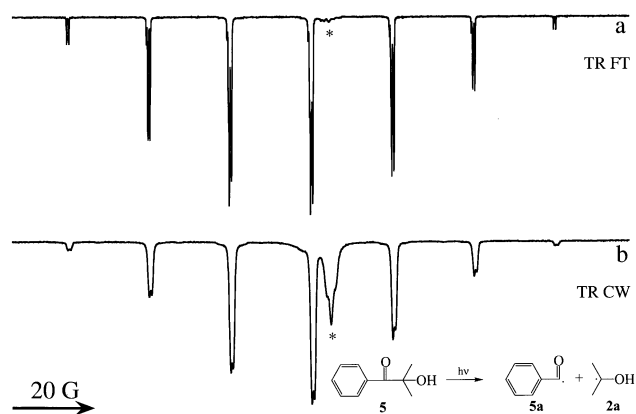
Fig. 4 (a) TR FT EPR spectrum recorded 400 ns, and (b) TR CW EPR spectrum recorded 300–600 ns following laser excitation (308 nm) of 2.4 M of 5 in an argon-saturated propan-2-ol solution at 297 K. The asterisk signifies the benzoyl radical 5a .
