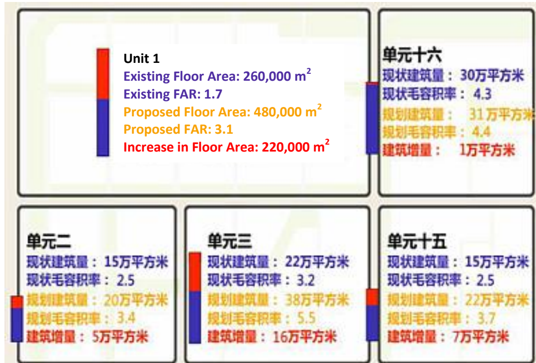
Figure 8 the density control of each redevelopment unit
