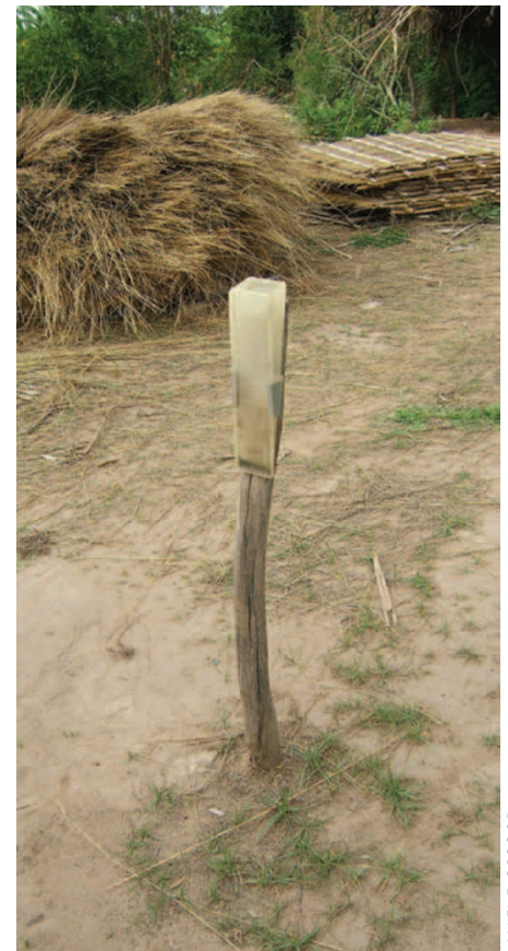
Manual rain gauge in Adi Ha, Ethiopia in 2009. This gauge is used as part of the validation for an index insurance project that also incorporates remote sensing data of rainfall at a location where there are very few ground-based rainfall measurements.
