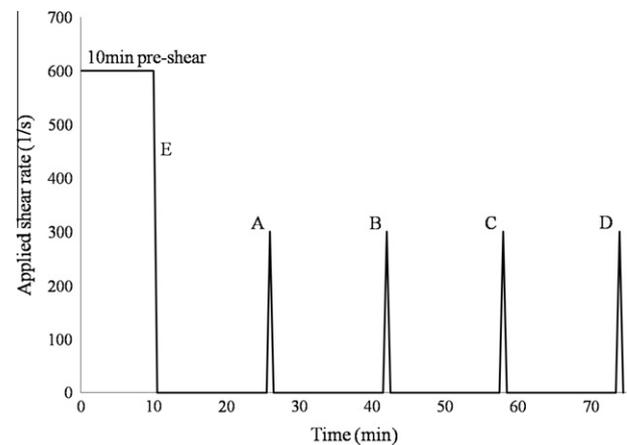
**Fig. 8.** Applied shear rate for SRE protocol.
