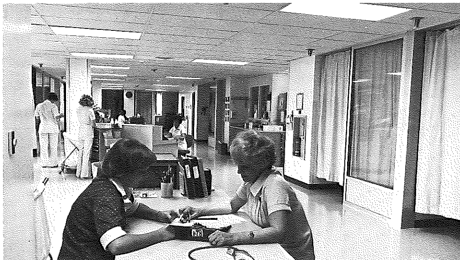
Light-colored, matte-finished surfaces in this hospital minimize glare.
