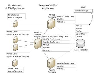
Figure 1: How Layers, Repositories and VLFSs Fit Together
